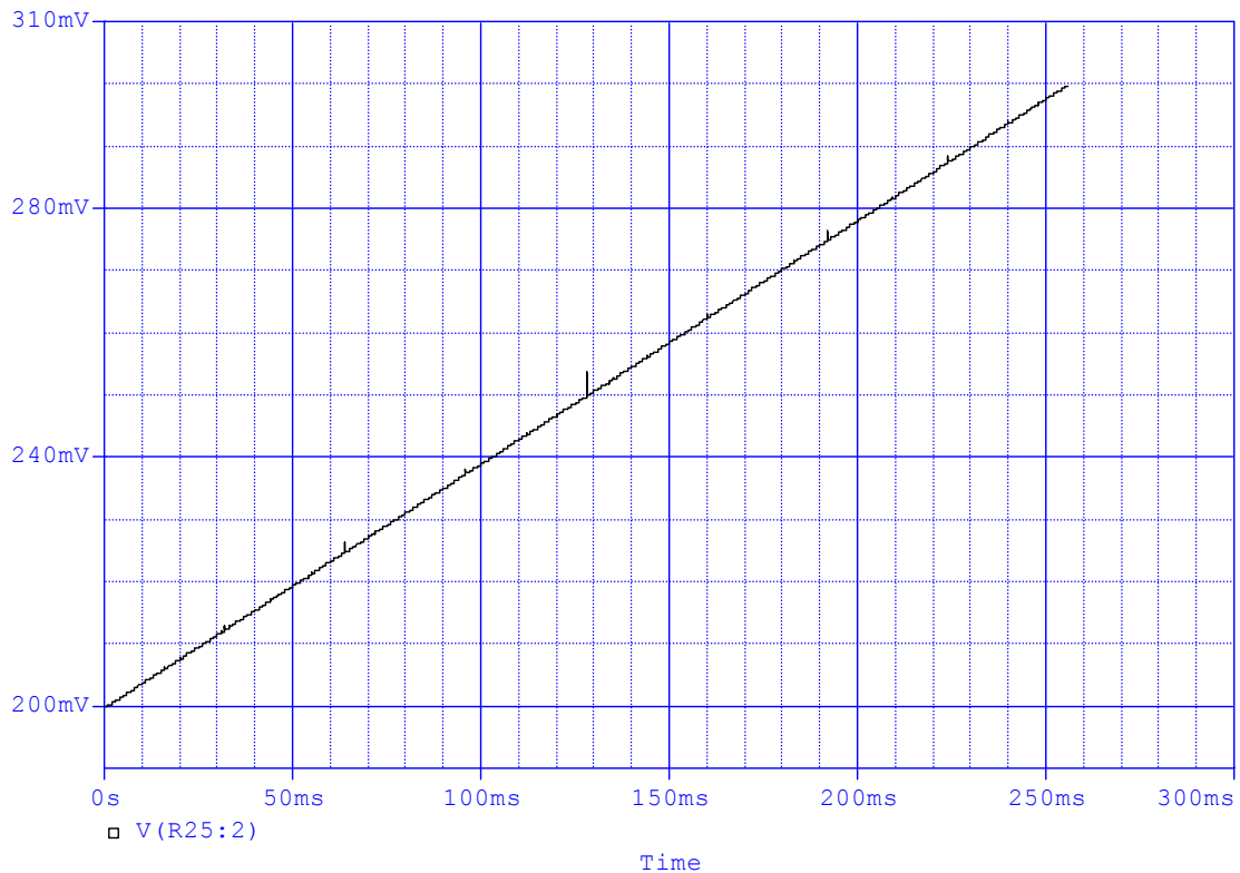
Figure 7. Subranging R2R DAC Simulation Results.
